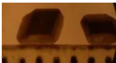
Figure 1 - \alpha -L-glutamic acid crystal obtained by slow evaporation method.
