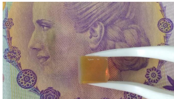
Figura 1. Extraction process: a gel with the silver nanoparticles is rubbed on the banknote surface.
