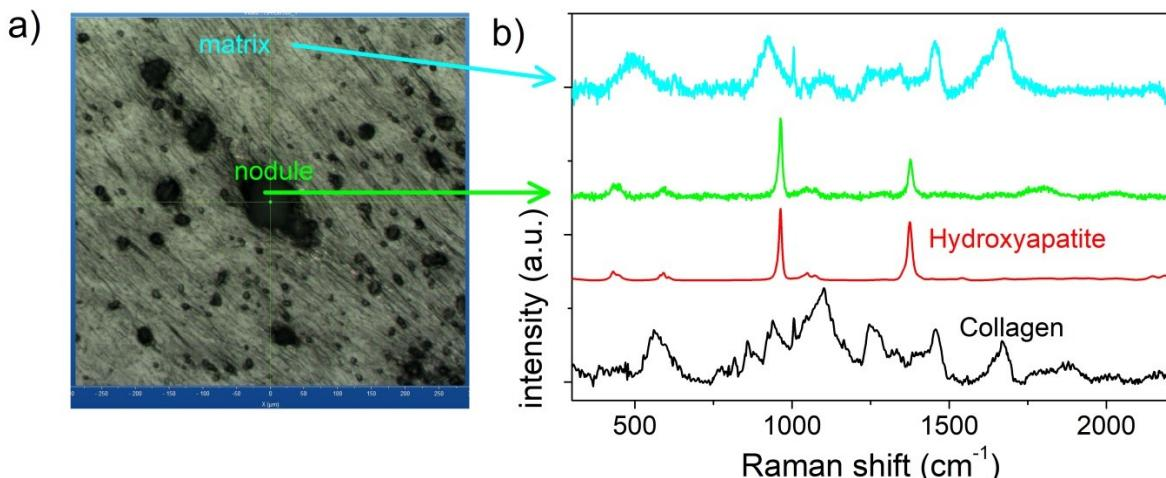
Fig.1. Nanoparticles-incorporated cells (a) showing HA nanoparticles nodules and Raman spectra (b) measured at nodules (green line), biostimulated cell matrix (cyan line) and reference spectra of hydroxyapatite (red line) and collagen (black line).
