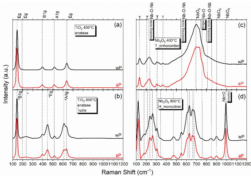
**Fig. 1:** Raman Spectra of  $TiO_2$  and  $Nb_2O_5$  at; (a) and (c)  $400^{\circ}C$ ; (b) and (d)  $800^{\circ}C$ , respectively. wP=without PAHT; aP=after PAHT
