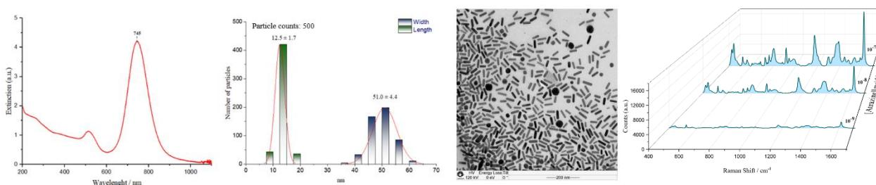
Figure 1. (a) AuNRs extinction spectra with its plasmon band maximum on 745 nm. (b) Width and length distribution of the AuNRs synthesized. (c) TEM micrography of the AuNRs. (d) Average SERS spectra of atrazine for different concentrations ( $10^{-7}$  to  $10^{-9}$  mol L<sup>-1</sup>).
