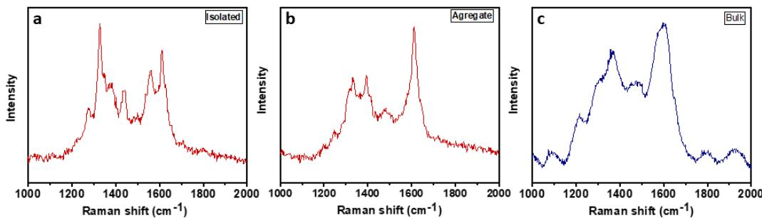
Figure 1. (a) TERS spectrum of an isolated CQD. (b) TERS spectrum of a small aggregate of CQDs. (c) Confocal Raman spectrum of the CQD's bulk sample.
