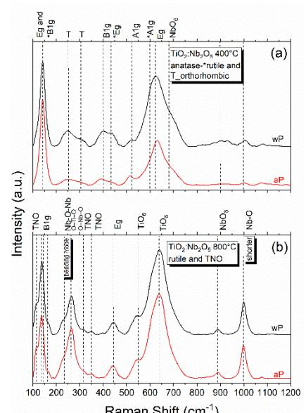
**Fig. 2:** Raman Spectra of  $Ti:Nb$  at: (a)  $400^{\circ}C$ ; and (b)  $800^{\circ}C$ . wP=without and aP=after PAHT
