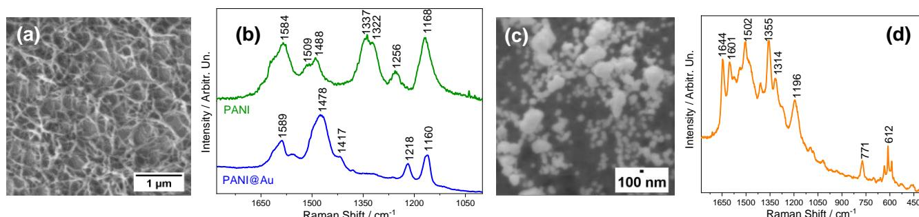
Figure 1. (a) PANI nanofibers MEV image, (b) Raman spectra of PANI and PANI@Au films, (c) PANI@Au MEV image, and (d) SERS spectra of R6G dye. ( $\lambda_0 = 632.8$  nm)
