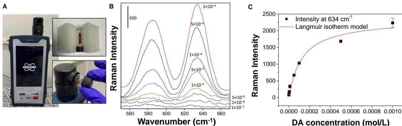
Figure 1. (A) Handheld Raman spectrometer and magnetic separation process before measurement. (B)  $550$  –  $670 \text{ cm}^{-1}$  range SERS spectra of various DA concentrations-AuMNP suspensions. (C) Langmuir isotherm model plot on experimental data from (B) at  $634 \text{ cm}^{-1}$ .
