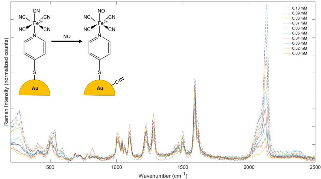
Figure 1 - SERS spectra of  $[\text{Fe}(\text{4Mpy})(\text{CN})_5]^{3-}$  upon interaction with different concentrations of NO.
