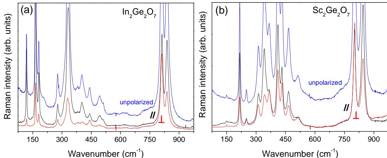
**Fig.1:** Polarized Raman spectra of (a)  $\text{In}_2\text{Ge}_2\text{O}_7$  and (b)  $\text{Sc}_2\text{Ge}_2\text{O}_7$  sintered ceramics.  $A_g$  modes are favored in parallel configuration (black curves), while  $B_g$  modes are enhanced in perpendicular light (red curves). The unpolarized spectra are shown in blue.
