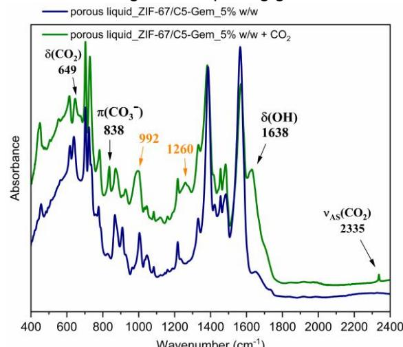
**Figure 2.** ATR-IR spectra in the region from 400 – 2400 cm<sup>-1</sup> for ZIF-67/C5-Gem porous liquid before and after CO<sub>2</sub> adsorption.
