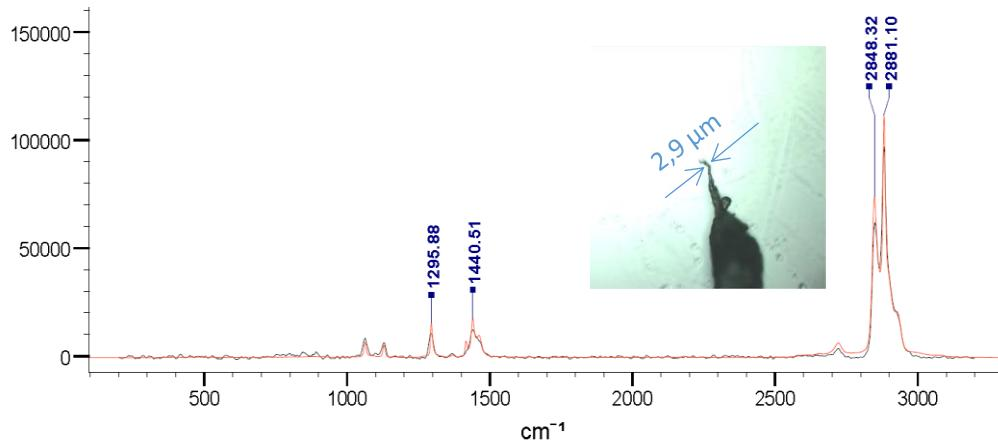
**Figure 1:** Raman spectra of a low density polyethylene microplastic compared to reference spectra. Measured spectrum (black line) and reference spectrum (orange line). Inset: sample picture indicating the measured region.
