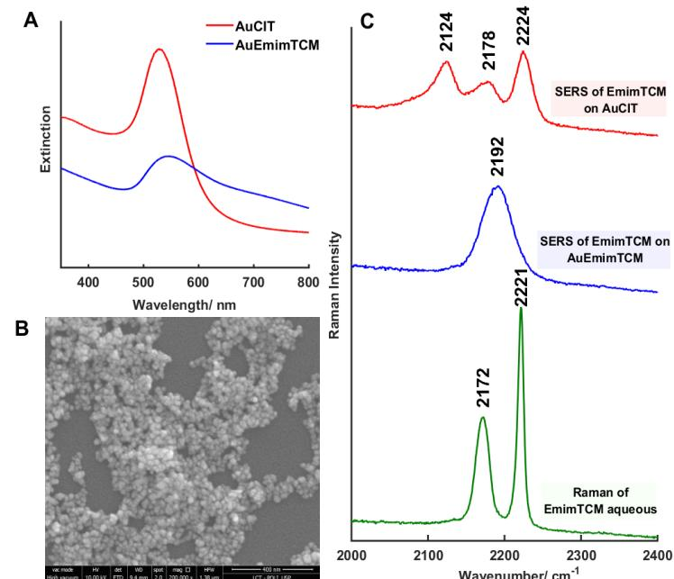
Figure 1. A) Extinction spectra of AuCIT and AuEMimTCM; B) SEM image of AuEmimTCM and C) Raman spectra of IL aqueous (green), SERS spectra of EmimTCM on AuEmimTCM (blue) and of EmimTCM on AuCIT (red).
