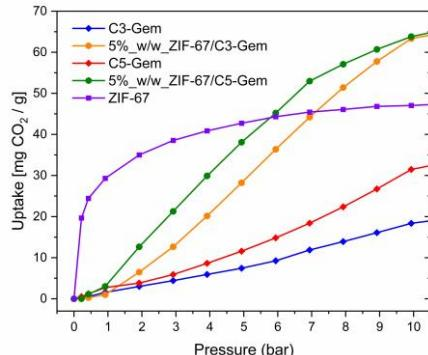
**Figure 1.** CO<sub>2</sub> sorption isotherms at 35 °C for materials studied. Blue line, C3-Gem; orange line, ZIF-67/C3-Gem, red line, C5-Gem; green line, ZIF-67/C5-Gem, and purple line, ZIF-67.
