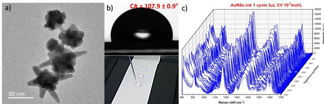
**Figure 1. a)** Au NSs TEM images. **b)** CA angle measures, and **c)** SERS spectra of CV on the Au NSs substrate.
