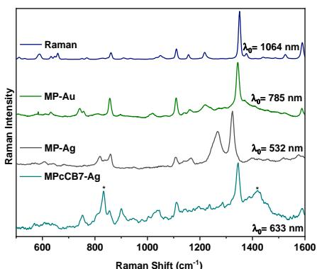
**Figure 1** – Raman and SERS spectra of methyl parathion with Au, Ag, and inclusion complex. \*CB7 modes.
