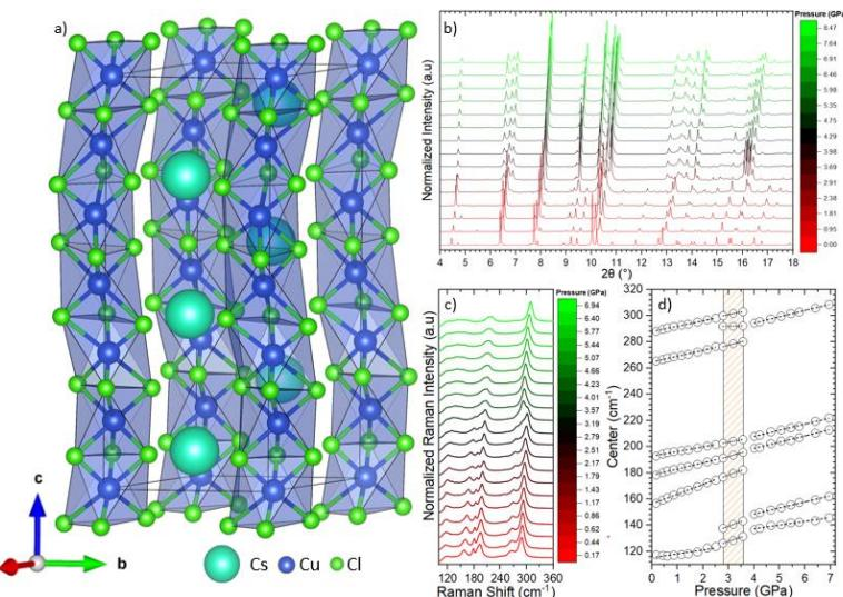
**Figure 1:** a) Room-temperature crystal structure of the  $\text{CsCuCl}_3$  ( $\text{P}6_5\text{2}2$ ), b) x-ray synchrotron diffractograms, c) the Raman spectrum and d) Raman modes evolution under high-pressure.
