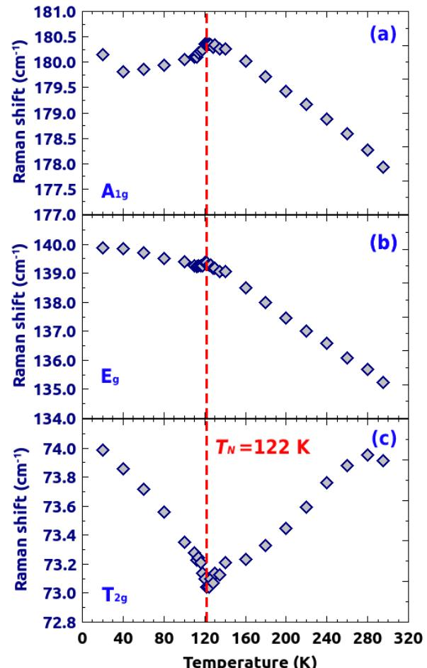
Fig1:  $\text{Cs}_2\text{AgBiBr}_6$  perovskite Raman modes centers as a function of temperature
