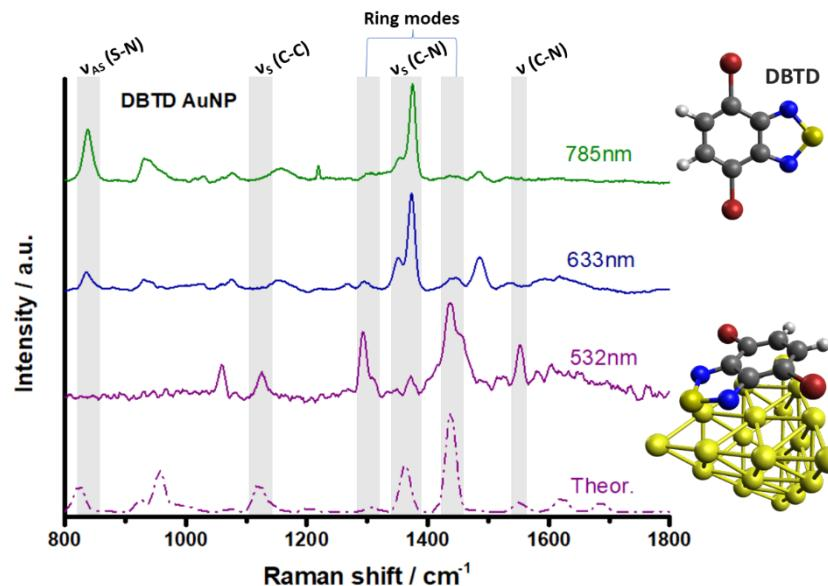
Figure 1 Experimental and theoretical SERS spectra of DBTD in AuNP in different excitation lines and multiconfigurational simulation of the 532nm spectrum.
