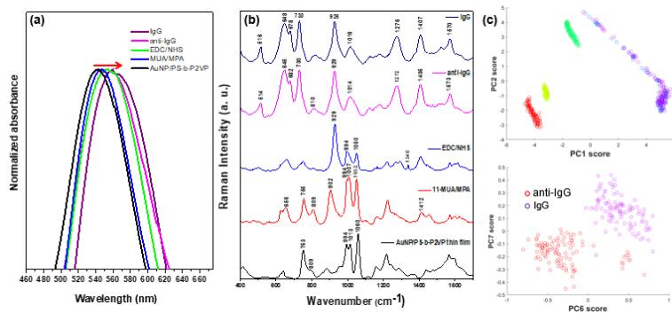
**Fig. 1** - (a) UV-vis spectra of each step of the substrate functionalization, (b) Mean SERS spectra of each step of the substrate functionalization and (c) Binary scatterplot of the PC1 × PC2 scores of the substrate functionalization and PC6 × PC7 scores of anti-IgG and IgG spectra.
