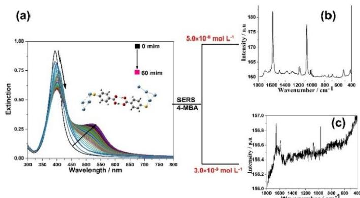
**Figura 1.** (a) Evolution of UV-Vis spectra of AgNP/4-MBA ( $5.0 \times 10^{-7}$  mol L<sup>-1</sup>) in pH=4 as a function of time and averaged SERS spectra of concentrations: (b)  $5.0 \times 10^{-8}$  mol L<sup>-1</sup> and (c)  $3.0 \times 10^{-9}$  mol L<sup>-1</sup>.  $\lambda_0 = 633$  nm.
